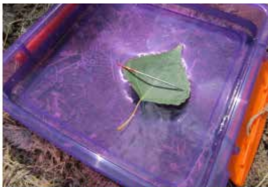
Needle pointer floating on a leaf in a camping food container
