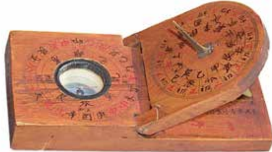
This Chinese navigating tool has a compass in its wooden base and a hinged sundial. The sundial has a folding gnomon on top and a hinged support underneath that can be put in one of 13 notches in the base to change the angle of the sundial.
